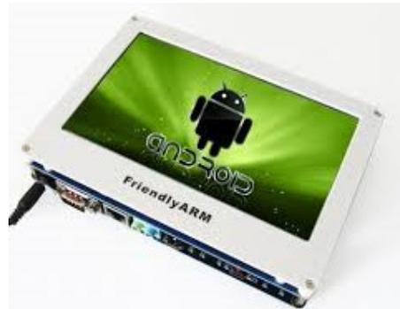
**Fig. 5.** Android booted on ARM board.
